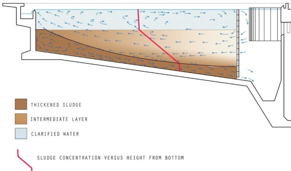
**Figure 1 - The hydrodynamic field (represented by the arrows) and the sludge concentration in a circular SST**
