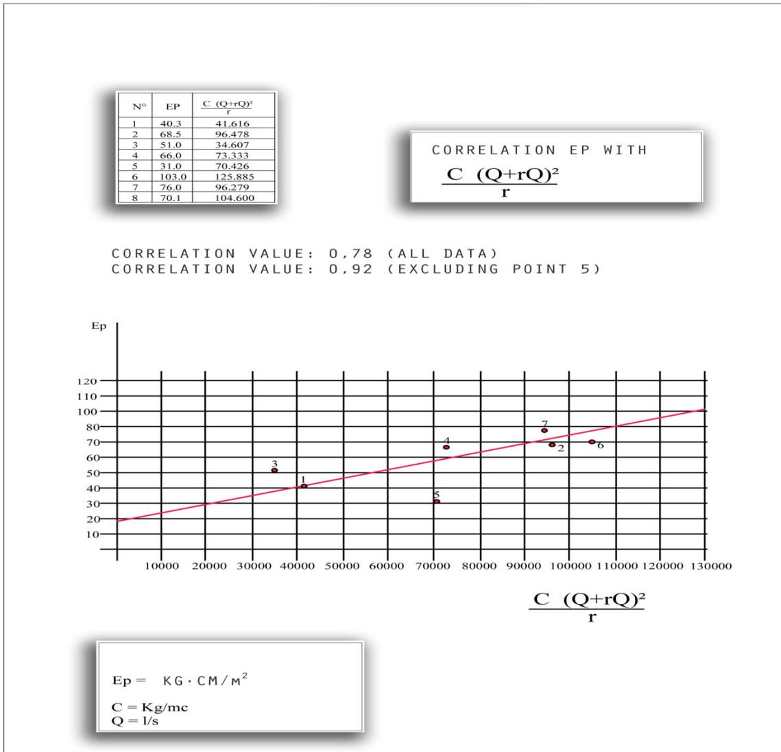
**Figure 2 - Correlation between the potential energy of the sludge blanket and the expression:  $C/r * (Q+rQ)^2$**
