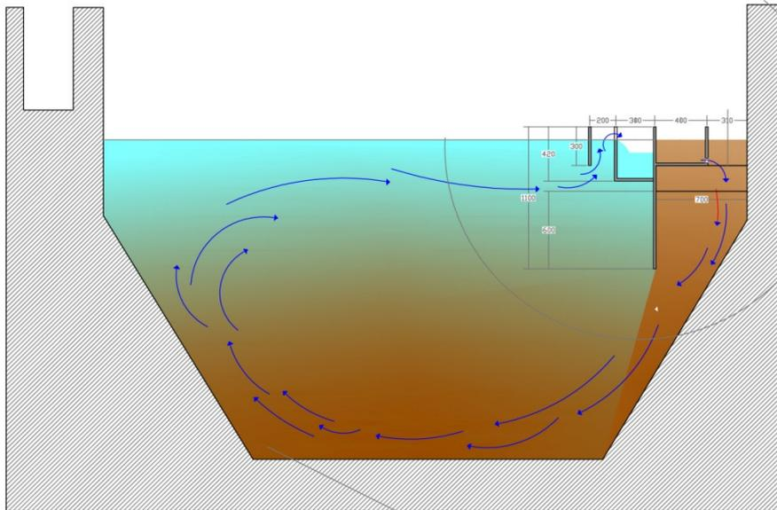
**Figure 4 - Cross section of a rectangular clarifier with longitudinal distribution of incoming MLSS for the entire length of one of the two long sides**
