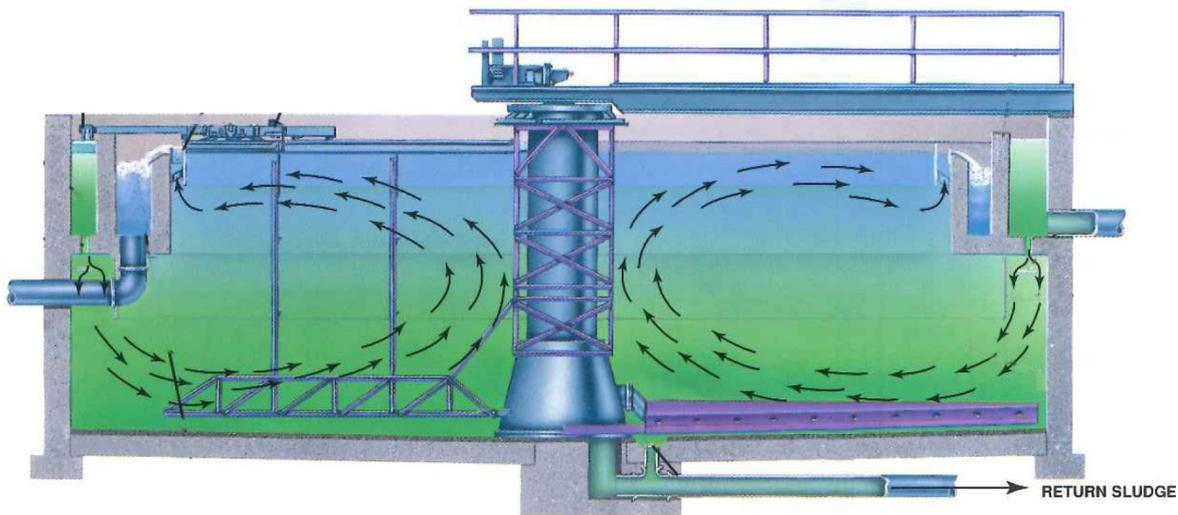
**Figure 3 - The hydrodynamic field (represented by the arrows) in a peripheral feed decanter**
